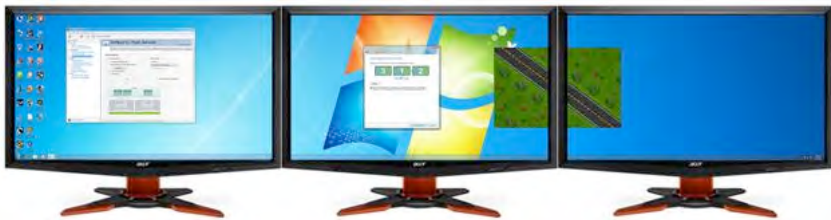
Figure 8: The two halves of the road image will move up and down as the pixel width is adjusted in the dialog. Be sure to align the images on both sides of the center display to ensure bezel correction is properly configured.
