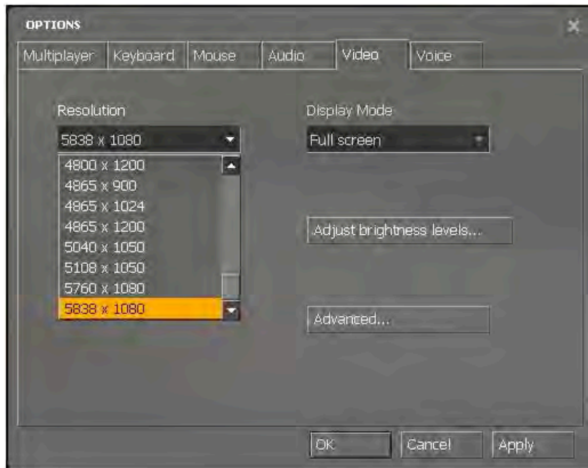
Figure 9: When you enable bezel correction, a bezel-corrected version of each 3-wide display resolution is added to the list of available resolutions - both within games as well as within the NVIDIA Control Panel. In the game settings above, the bezel corrected resolution would be the larger 5838x1080 resolution.
