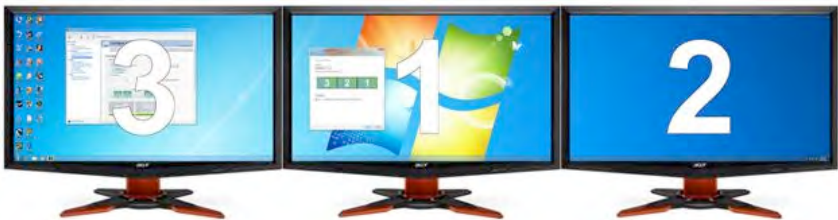
Figure 4: You will see numbers appear on all three displays when the Identify button is pressed. This is the numbered arrangement you need to make your desktop work correctly.
