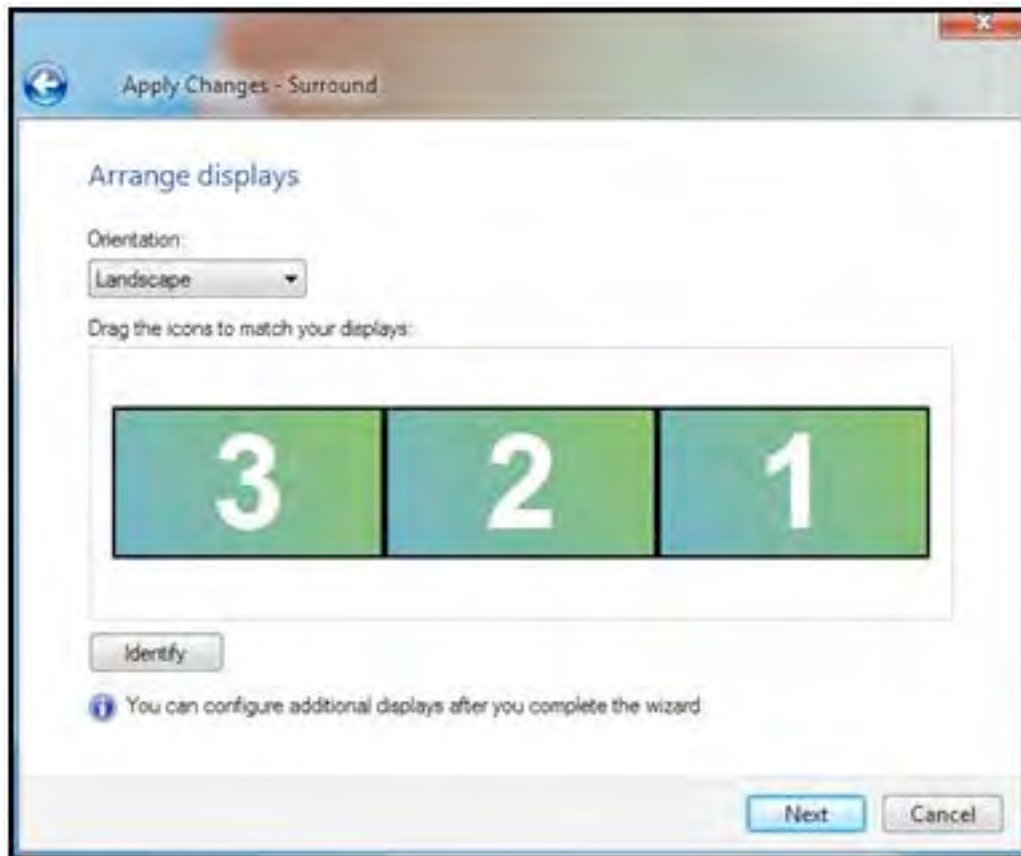
Figure 3: Click the Identify button to determine the correct numbered order for your displays.
