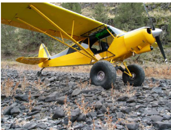
Very popular for bush flying is the Piper Super Cub with oversized tundra tires for rough fields.
