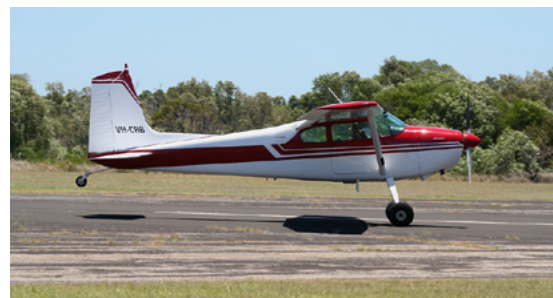
The more powerful C-180 tail surfaces are square-shaped and larger. This was later adopted for the C-170.
