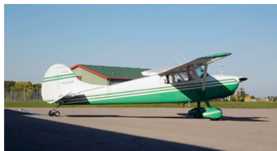
C-170 tail surfaces were originally round-shaped.
